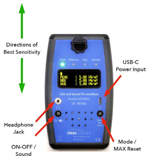
This sensitive meter is capable of measuring potentially harmful mmWave radiation from any continuous or pulsed digital sources. To help identify these various sources, the Safe and Sound Pro mmWave includes a built in speaker with adjustable volume levels. Each mmWave source has its own unique sound signature.
