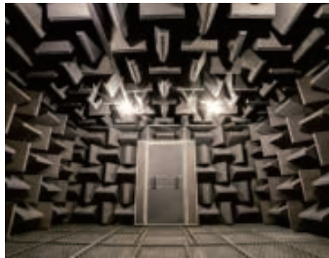
55m³ acoustic chamber with 100Hz effective cut-off frequency.
