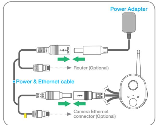
Figure 2: Connecting to power
