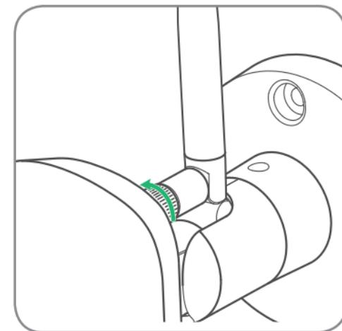
Figure 1: Attaching the antenna
