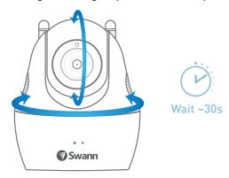
Once ready, the camera goes into Wi-Fi configuration mode and talks you through the setup process. Listen carefully and follow the voice prompts to complete the setup of the camera.
