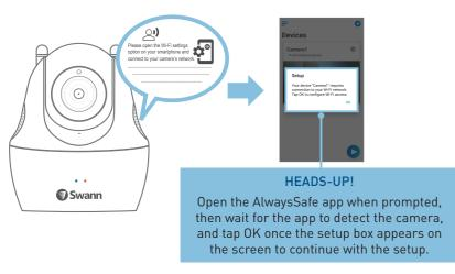
**Note:** The camera's Wi-Fi configuration mode times out in 10 minutes. Simply restart the camera if you need more time to set it up.
