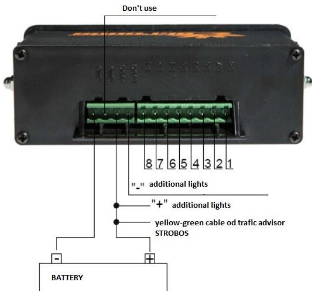
The traffic advisor should be connected to a siren or directly a battery. Connecting the lamp to another power source may result in its damage or the level of light intensity will be insufficient for proper operation.
