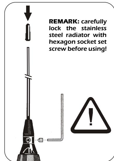
**REMARK:** carefully lock the stainless steel radiator with hexagon socket set screw before using!
