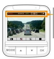
The status bar at the top of the screen instantly provides you with information about video resolution, available recording time, GPS connectivity, active features, and memory card & battery status
