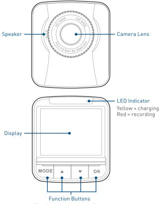
Use these buttons to perform operations corresponding to the icons displayed on the bottom of the screen
