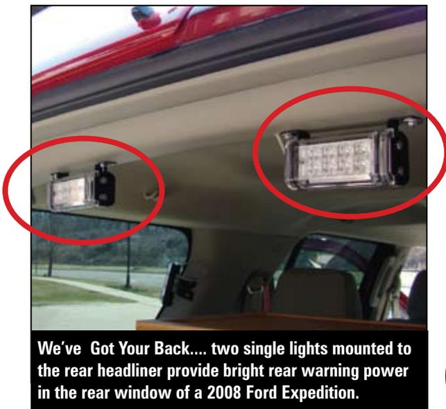
We've Got Your Back.... two single lights mounted to the rear headliner provide bright rear warning power in the rear window of a 2008 Ford Expedition.
