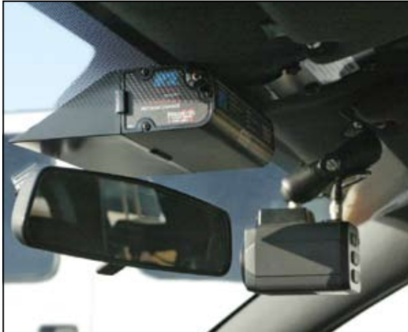
Permanent Headliner Mount positions light above rearview mirror without obstructing the mirror.
