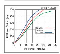
Figure 8 — RM Italy BLA600 input power versus output power.
