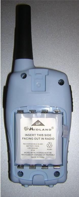
Remove the belt clip (pull spring and remove to top) and open the battery compartment.
