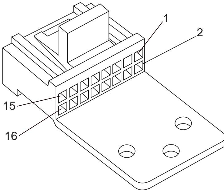
**Figure 19: Pin Configuration of Rear Accessory Connector (as viewed from the rear of the radio)**
