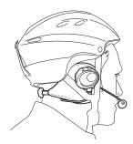
If your helmet is not equipped with the two removable pads, you could anyway mount your **BTSKI** system by using the supplied Velcroband. Be sure to fix the Velcro-band as shown in the figure.
