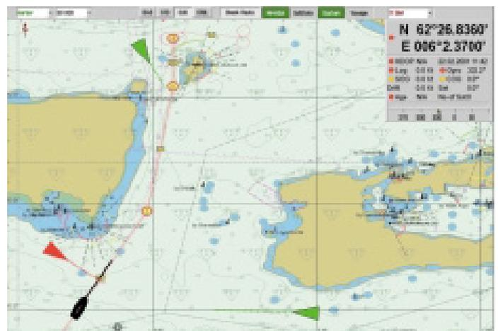
*Vessels posing the potential risk of a collision are shown in red. Vessels passing safely are shown in green.*
