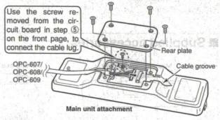
⑤ Connect the supplied flat cable\* and ground cable (coming from the RMK-2) as shown below.
