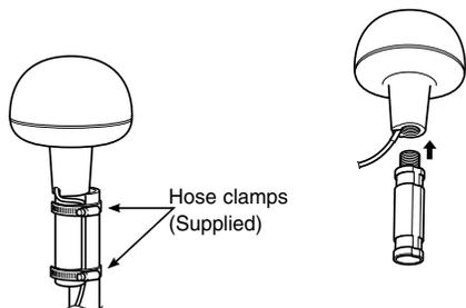
The supplied extension pipe is to be inserted firmly into the base of the GPS receiver and screwed in a clockwise direction.
