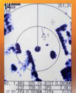
10 targets can be plotted on the screen and follows the motion of the other ships.
