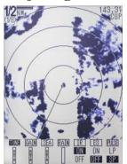
Changing the settings can be made quickly and easily. TUNE, GAIN and SEA are adjustable automatically or manually.
