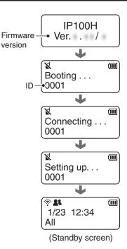
Rotate [PWR/VOL] to turn ON the power.
