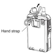
To facilitate carrying the communication terminal, slide the hand strap through the loop on the top of the rear panel, as illustrated to the left.
