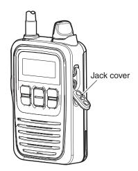
Be sure to turn power OFF before connecting or disconnecting optional equipment to or from the  $[\mathscr{N}/ \ensuremath{\Omega}]$  jack.
