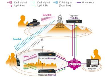
IDAS receiver voting improves the talk back capability of IDAS handheld and mobile radios. The IDAS networked receivers (where IDAS repeaters' transmission is inhibited and used as receivers) are distributed to the communication area. Each receiver receives a signal from a terminal radio and transfers it to the repeater site, and the repeater relays the best signal or transfers it to the remote dispatch. The UC-FR5000 has a built-in voting function, so an external voter device is not required.
