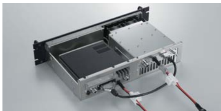
IC-FR5100H series has built-in power amplifier unit.
