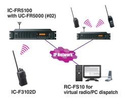
When using the IC-F3102D series in IDAS multi-site conventional mode, the IC-F3102D can communicate with other IDAS radio users working with other repeater sites and/or virtual radio/PC dispatch stations on the IDAS network.
