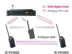
The IC-F3102D series can receive both analogue and digital mode signals on a single channel and automatically selects the received mode to reply to the received call, while the talk back timer remains. It's a smart way to grow into digital radio - at your own pace, as your budget and comfort allow.
