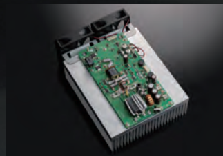
PA Unit with a Large Heatsink
