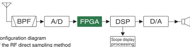
Configuration diagram of the RF direct sampling method
