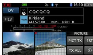
Enjoy the latest DV mode features with the IC-705. Have direct access to the D-STAR network with Terminal/Access point modes. Additionally, the IC-705 has the Photo Share feature introduced with the IC-9700. Share photos, without the need of a computer with other users.
