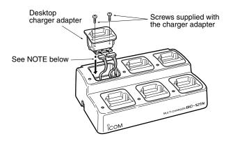
**NOTE:** Some of the PCB type desktop charger adapters do not need connection of the 3-pin connector.
