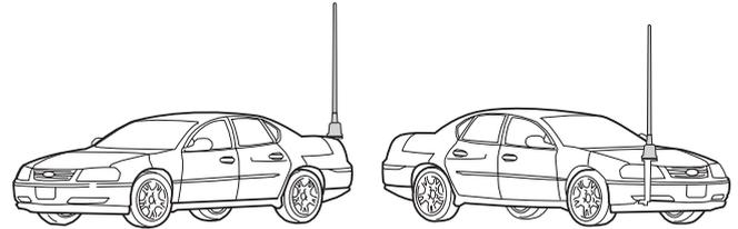
**NON-RECOMMENDED** installation methods use a Universal Gibbet Mounting System (both at the rear) shown on a typical minivan or 4WD vehicles. Note the entire Antenna Main Assembly and partially Whip Section are **OBSTRUCTED** by vehicle metal panels. Communications will be affected.
