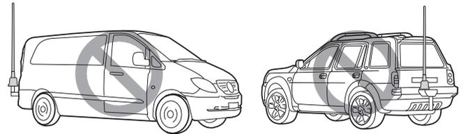
For best communications, position the antenna as high as possible. The Figure 1 shows the preferred option selection. The Figure 2 shows an antenna installation that uses the optional AH-5NV, for best communications on the 30–300km (18.6–186.5 miles) short ranges, and up to 1500 km (932 miles) medium ranges.
