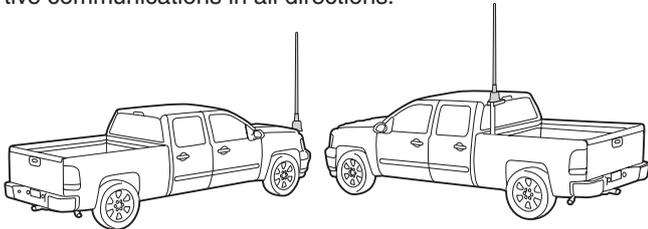
Recommended installation options on a typical sedan vehicle use a Universal Gibbet Mounting System for both front and rear antenna locations. Note the tuning antenna unit is optimally raised above the trunk and hood of the vehicle.
