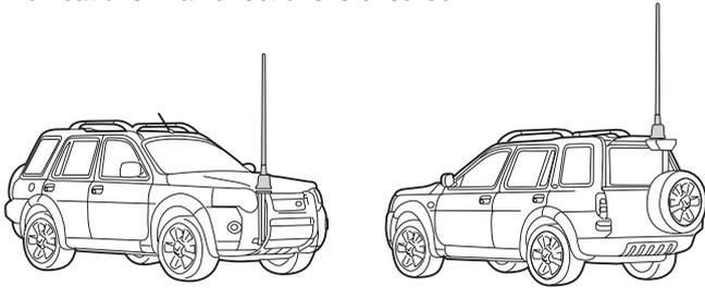
Recommended installation options on a typical pickup vehicle use a Universal Gibbet Mounting System (front) and a customer provided bracket (middle). Both methods provide effective communications in all directions.
