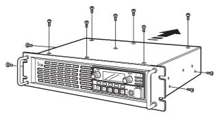
② Remove 3 screws from bottom and 2 screws each from both sides of the repeater.
