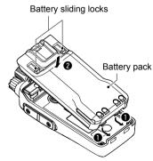
1. Push both battery sliding locks in the direction of the arrow. (11) The battery pack is then released.
