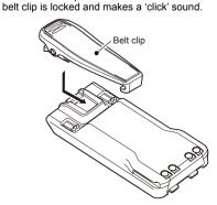
• Lift the tab up (1), and slide the belt clip in the direction of the arrow (2).
