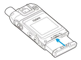
To remove the battery, turn off the product first. Push the battery latch to the bottom till the battery pops out, and then remove the battery.
