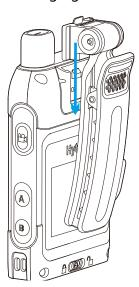
To remove the belt clip, do as follows. Toggle the metal dome, and then remove the belt clip upwards.
