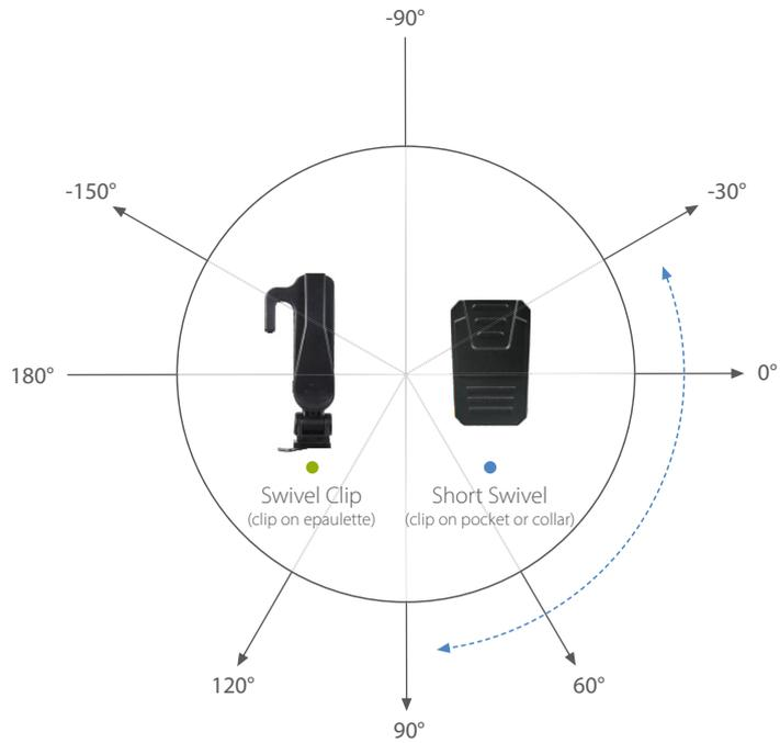
Adjust recording angle by rotating 30° every time, 360° maximum.
