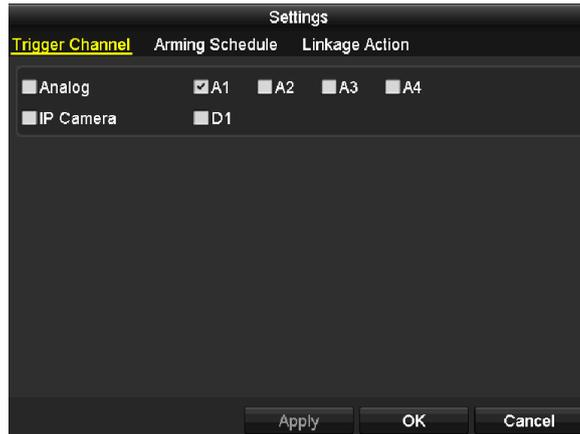
Figure 8. 140 Set Triggering Channel of VCA Alarm
