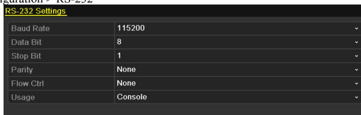
A screenshot of the RS-232 Settings interface. The title is "RS-232 Settings" in yellow. Below it is a table with two columns: the parameter name and its current value. Each row has a small downward arrow on the right side, indicating that the values can be changed.
