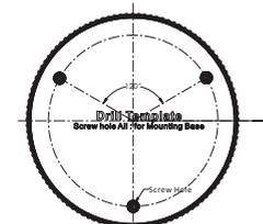
Figure 2-1 The Drill Template
