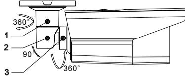
Figure 2-7 3-axis Adjustment
