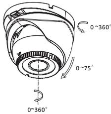
Figure 2-4 3-axis Adjustment
