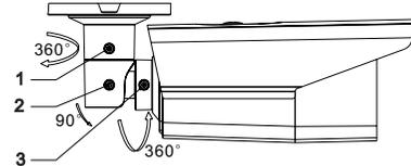
Figure 2-7 3-axis Adjustment
