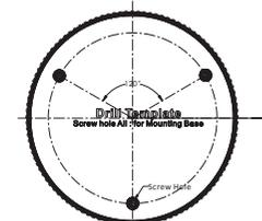
Figure 2-1 The Drill Template
