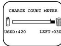
After 450 cycles, at switch on the radio will emit a series of long beeps, and on LCD models the message will change to **BATTERY COUNT EXCEEDED REPLACE BATTERY**. The radio will continue to operate but its operational time may be reduced, eventually failing all together.
