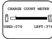
The warranty on all batteries is 12 months or 450 charge cycles, whichever is the sooner. After 420 cycles, at switch on the radio will emit a series of short tones, and on LCD models a waste bin icon will flash to alert you to the need to buy a new battery.
