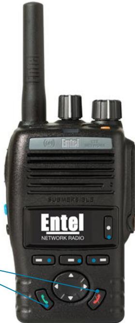
The Green and Red buttons can be used to setup and end polite calls instead of the soft keys shown in Fig. 10
