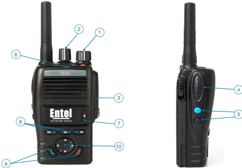
1. On/Off/ Volume control. Rotate clockwise to turn ON and increase volume. Rotate anti-clockwise to reduce volume & turn OFF.
