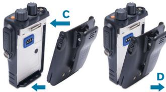
1. To attach (C), locate the pegs on the bottom of the battery into the slots on the radio and pull the 2 latches downwards, carefully pushing the battery into the radio. Release the latches ensuring the battery is full attached.
