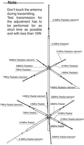
※If SWR is less than 2.0, you can operate the antenna tuner 'Through". (However, if protection circuit of the transceiver is operated and the transmitting is stopped automatically, it is not so.) Since CPVU8 is high shortening ration antenna, use the antenna tuner if changing the frequency.
