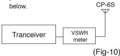
2 Adjustment procedure can be started from any frequency you like. Transmit at desired frequency and trim adjustment length of radial element to have lower VSWR at the frequency.
