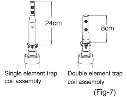
Single element trap coil assembly
