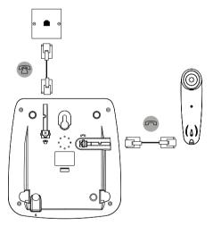
Plug one end of the handset curly cord into the socket marked on the underside of the base and the other end into the socket at the bottom of the handset.
