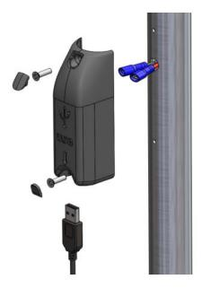
It is recommended that these units are fused individually with a 1Amp fuse (24V systems) or a 2Amp fuse (12V Systems).
