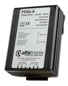
and a 12A (continuous), which overcome these configuration problems. The Alfatronix converters mimic the 12V battery and 12V ignition function by providing two outputs, either of which can provide full power. One output is available whenever the 24V battery is connected. The other output is switched by the 24V ignition switch. Now the ICE equipment can be fitted to the 24V truck as simply as fitting it to a 12V car.
