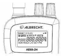
The display has indicators that show the scanner's current operating status. The display information helps you understand how your scanner operates.
