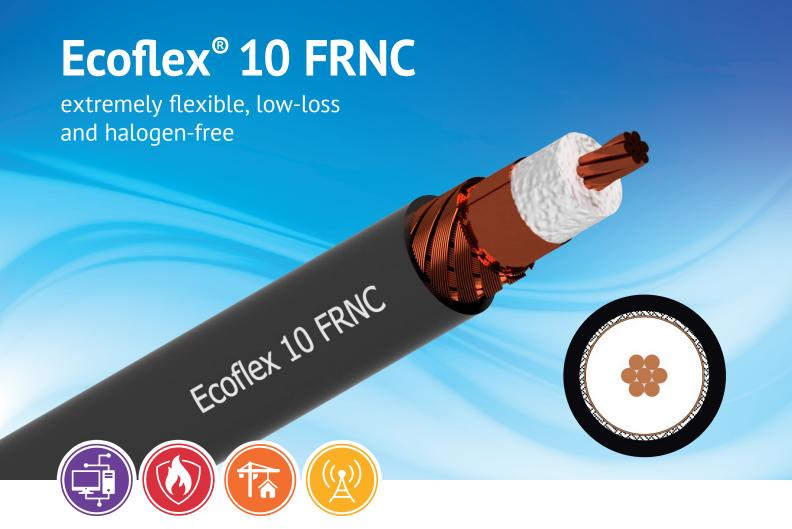
Ecoflex 10 FRNC is a flexible and very low-loss 50 ohm coaxial cable designed for the frequency range up to 6 GHz. State-of-the-art production methods and the use of a low attenuation PE-LLC dielectric with a gas content of over 70 % enable low attenuation values that set standards for flexible coaxial cables of this size.
