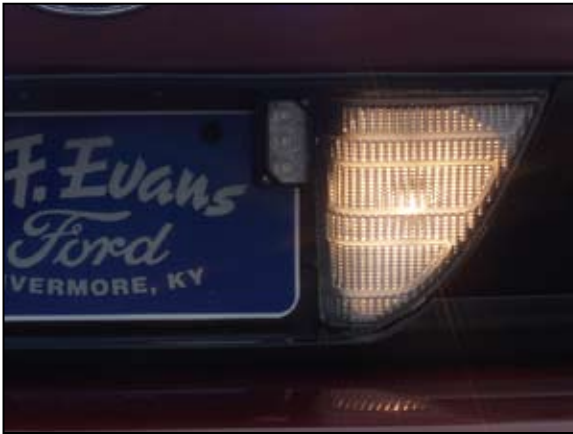
UnderCover™ Strobe Tubes can be used in the head lamp, tail lamp and turn signal applications.
