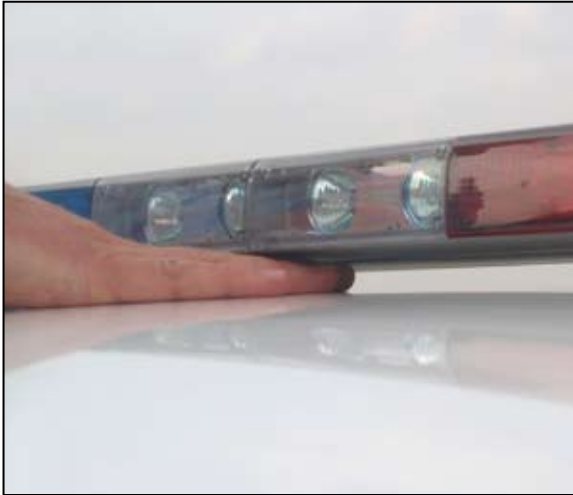
Low Profile Fixed Mount Brackets have a low clearance of just 3/4" on Ford Crown Victorias.
