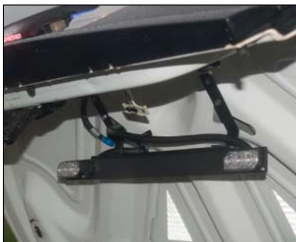
Dual function light offers a warning signal while the trunk is open. Ford Crown Victoria mount shown.
