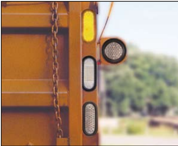
Recessed mount design can be used on all types of vehicles with a standard 4" round cutout.
