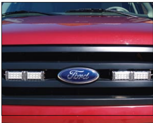
Two Dual Predator 2™ Lights installed in the front grille of a utility vehicle.
