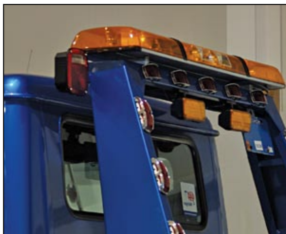
Amber lens MTL 2000 lightbar shown mounted on a tow truck. Bar has 2-center Work Light Modules.
