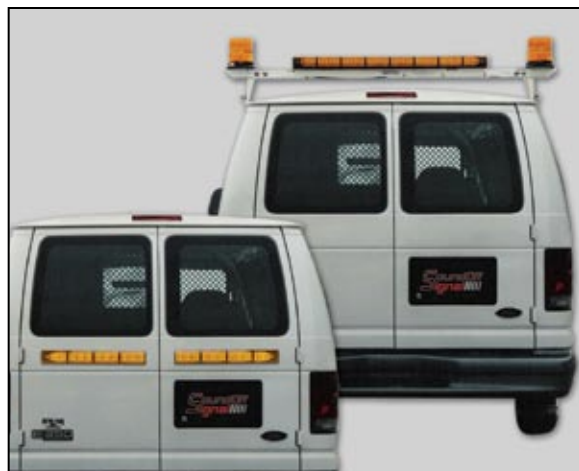
TrafficMaster Amber bars shown on utility/work vans offer additional safety for workers.
