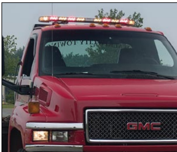
ETL 5000 Red & Amber LED lightbar shown on a Tow Truck. Adjustable Mount Brackets used.
