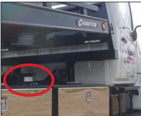
Light shown mounted under the bed of a tow truck with optional 90 Degree Bracket.
